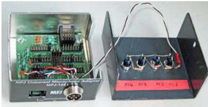
The four momentary push-button switches and four resistors are mounted in the lid of the MFJ-1251 metal case.
