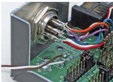
Close-up shows two wires from the case-lid switches soldered to the empty RJ45 modular jack position "J2", at the pin 3 and pin 6 locations. (Pin 1 is closest to camera.)
