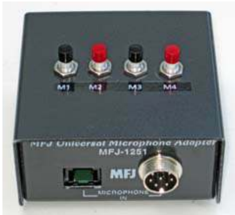
External keypad with the four memory buttons M1 - M4 suitably labeled.
