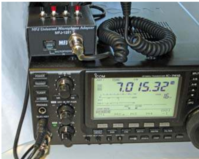
Ready for some CW! The external keypad based on an MFJ-1251 is shown in-line with the Icom HM-36 hand microphone and cabled to the Icom IC-7410 8-pin round MIC input at bottom left.
