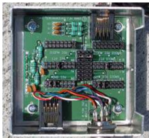
MFJ-1251 with modified jumper settings for an Icom 8-pin round microphone plug to an Icom 8-pin round MIC connector.
