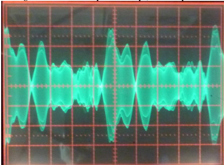
Figure 17: 100W PEP speech envelope, 6 dB compression.
